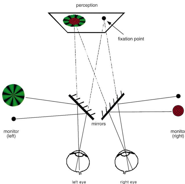
Fig. 1. Schematic diagram of the experimental setup. In this example, the stimuli were centered on the left eye's blind spot. During the experiment, observers usually experience rivalry between the green radial grating and the red circular grating. Their task was to track and record the appearance and disappearance of right eye's small red target.
